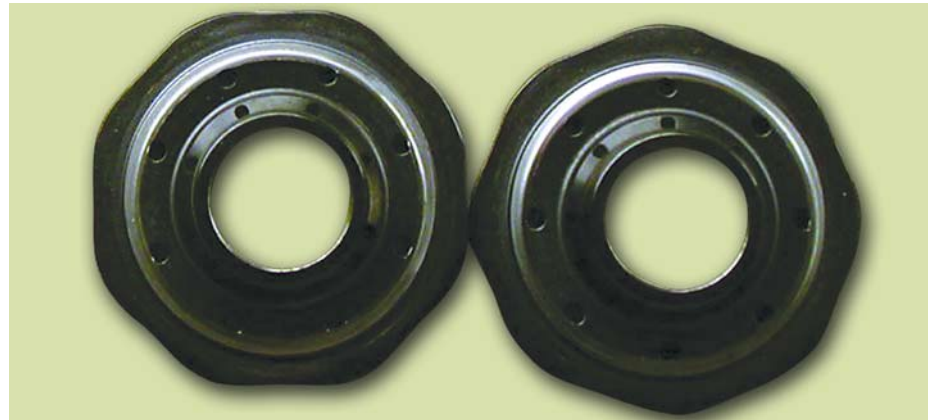
Figure 1. Titanium intake valve spring retainers with two microns of Carbon Raptor, shown after the Homestead 400. Carbon Raptor is intact on the spring loading surfaces. Coating breakthrough and some wear occurred on the damper contact surface.
