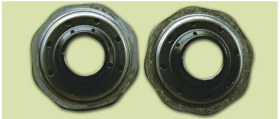
Figure 2. Titanium exhaust valve spring retainers with two microns of Carbon Raptor, shown after the Homestead 400. Breakthrough of the coating was seen on the outer spring flat, and with no loss of dimension. No damage to the Carbon Raptor coating occurred on the inner flat. Some wear occurred on the damper contact surface.
