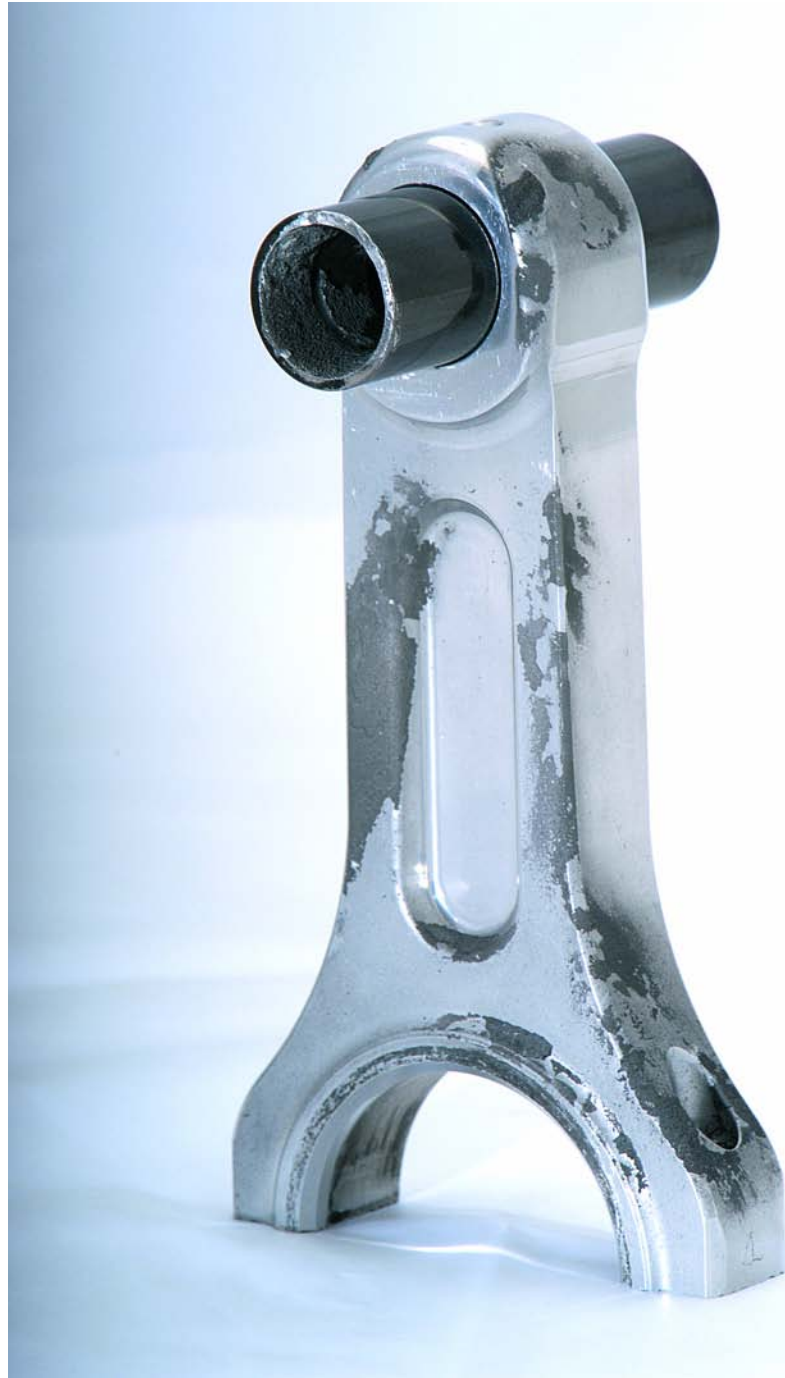
Figure 1. A Carbon Raptor coated piston pin that saved an engine block in a blown alcohol drag racing application. Parts courtesy of Quest Racing, Worcester, Massachusetts.
