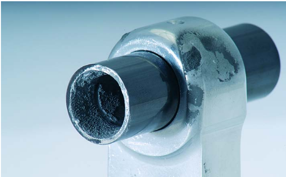
Figure 2. A close up of the piston pin in small end of a connecting rod. Parts courtesy of Quest Racing, Worcester, Massachusetts.
