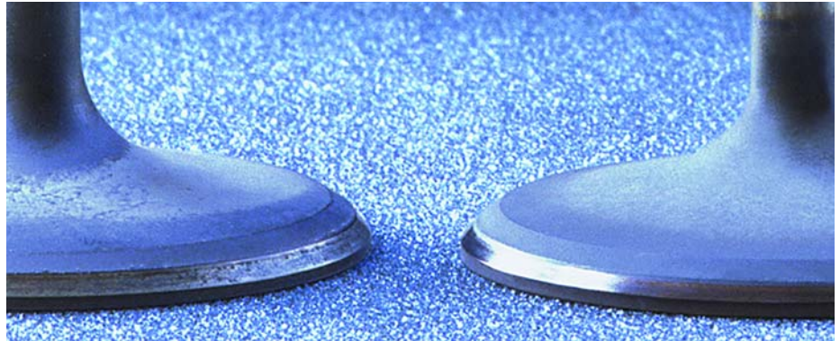
Fig. 1 – Identical valves, run under identical conditions. Uncoated on left, coated on right.
